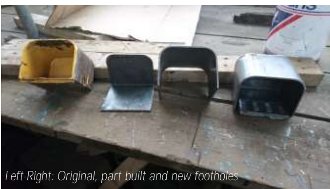
Repairs to Secondman's side, with new foothole and lamp bracket fitted.
